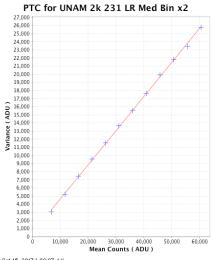
Oct 15, 2017 | 09:07 AM Gain: 2.3837 e-/ADU Std Dev: 1.6866 ADU Noise: 4.0203 eTwo typical photon transfer curves are shown. As with earlier 42-40 devices the photon transfer curves were considerably more linear at a binning of 2x2 pixels compared to no binning, a well-understood effect of charge repulsion between electrons of neighboring small pixels. I verified that the linearity of counts versus time is good, about 1% over the full dynamic range.
