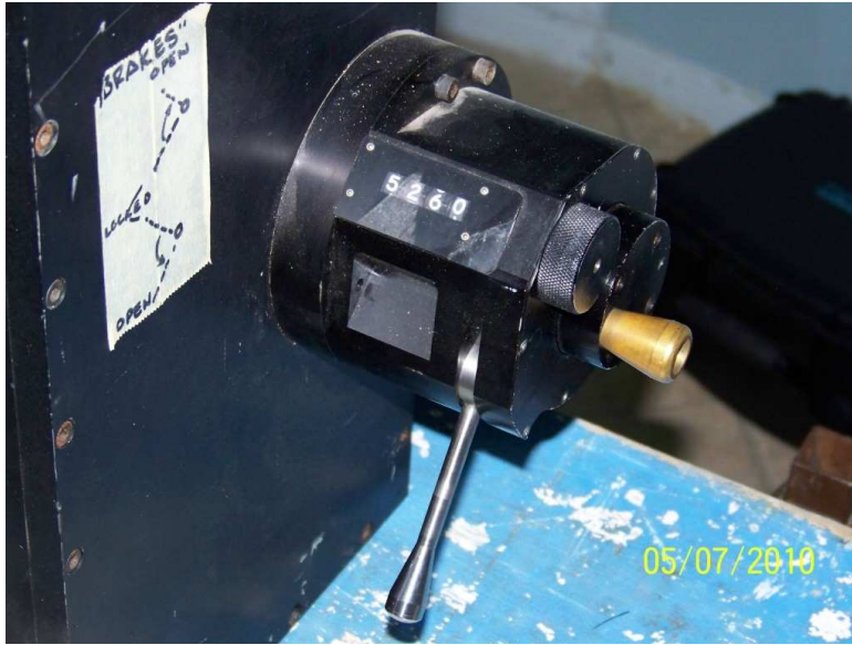
Figure 2.8: Crank that correlates the angular value of \gamma with a numerical code.
