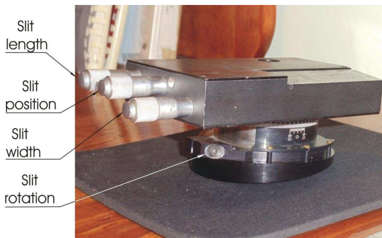
Figure 2.6: Micrometers used to set the slit length, position and width. The screw allows to set the rotation angle.
