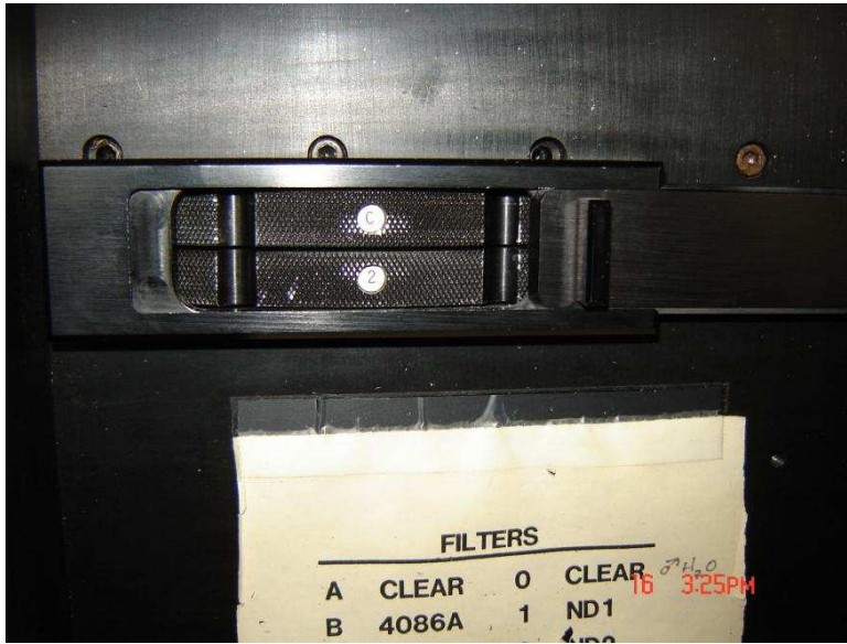
Figure 2.7: Filter wheels window at the rear side of the spectrograph used for selecting the desired interference filter.
